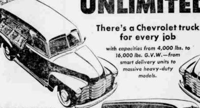
LIGHT-DUTY CANOPY EXPRESS Model 3107-116 inch wheelbass Maximum G.V.W. 4600 lbs. Also available in Medium Duty Model 3807 — 137 - inch wheelbase, Maximum G.V.W. 6700 lb.
