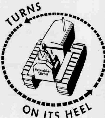
The heavy-duty steering clutches permit this tractor to make a full circle turn... directly on its heel under load. The turning radius of the Diesel D2, for example, is only 5'7"... a big advantage for working in narrow quarters or short headlands.
