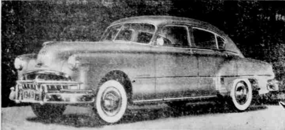
This is the four door deluxe Pontiac sedan in the Streamline series. Forward thrust has been gained by lowering the hood. Body contour is in the modern manner and yet unmistakably Pontiac. Added safety is compounded by reduced pillars and a curved windshield which gleaming sweep has been increased nearly six inches. Both Pontiac Streamliner and Pontiac Chieftain lines use a 120 inch wheelbase and Hydra-Matic transmissions optional at extra cost.
