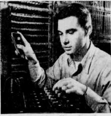
2. While you sleep this new electronic tester is at work . . . combing over circuits to see if it can spot a "leak" in the office or out on the lines. For even the best-insulated cables now and then allow moisture from rain or fog to creep in. By recording current loss on the lines, the tester checks loss of efficiency that might mean future trouble.
