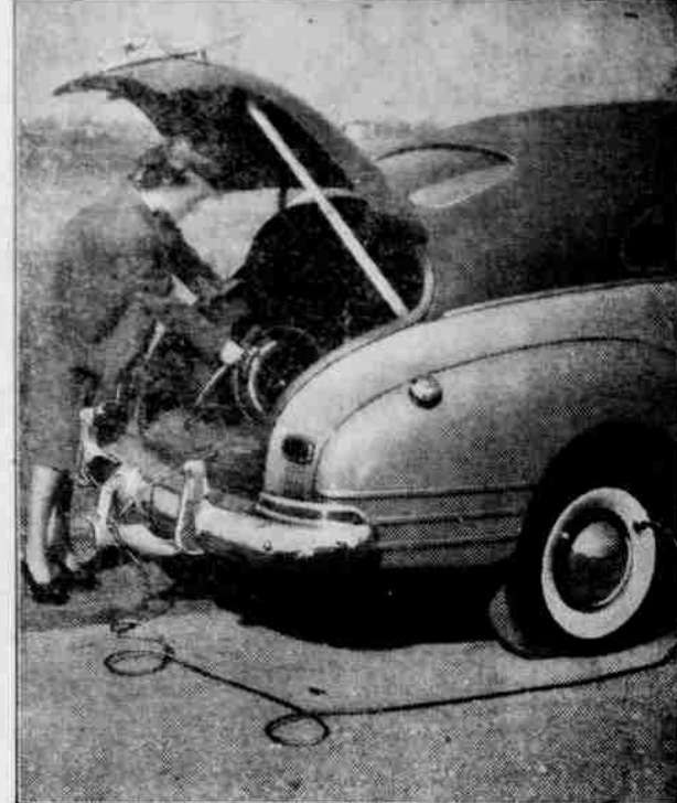
Latest entry in the "what-won't-they-think-of-next" sweepstakes is the handy gadget illustrated here, euphemistically known as "Spare-Aire," a Chevrolet accessory. Designed to "steal" air from the spare tire to inflate a punctured or slowly leaking flat, this accessory eliminates tire-changing when within reasonable distance of a service station. Since approximately 90 per cent of all flat tires have leaks so slow that an emergency inflation will suffice, the new inflator will eliminate most roadside tire changes. It will pipe half the air from the spare, and a few pounds from each of the other tires, if necessary. Women drivers, especially, will appreciate this new convenience.
