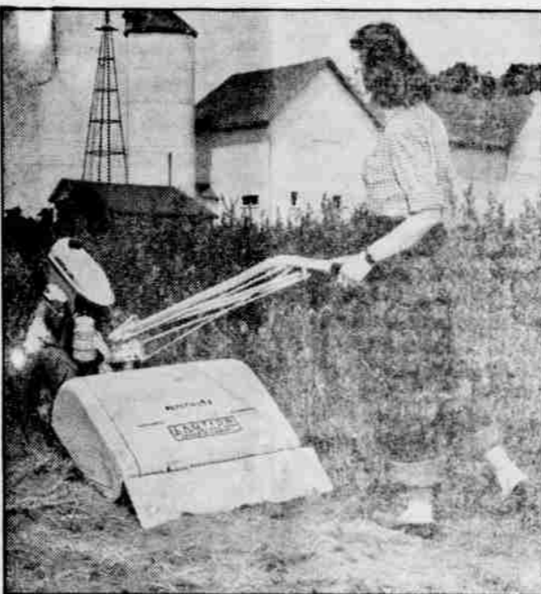
The new Rototiller farm machine, produced by Graham-Paige Motors in the giant Willow Run plant, prepares soil for planting in a single operation, making unnecessary the three operations of plow, disk and harrow. The five-horsepower tillage unit, which churns and crumbles the soil to a depth of nine inches, has attachments which adapt it to a score of other farm tasks such as bulldozing, seeding, mowing, snowplowing and other operations.
