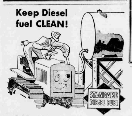
Every drop of fuel your Diesel burns must go through injector-nozzle holes no larger than a human hair. Even tiny dust specks may jam those holes! To help make present in-jectors last, kcep your Standard Diesel Fuel clean. Store supply tanks under cover. Make sure all bungs, fill caps, etc., are tight. Use filters when filling tractor or equipment tanks. You'll find 100% clean Standard Diesel Fuel uniformly dependable.
