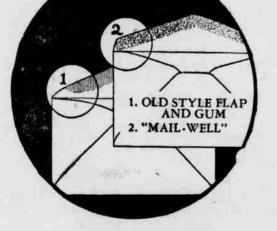
Notice in the above illustration the entirely different construction of the two envelope flaps. Figure 1 shows the old style flap. Figure 2 shows the "Mail-Well" flap which has been designed to protect the contents of the envelope. The outstanding advantages of this special high shoulder flap are:
