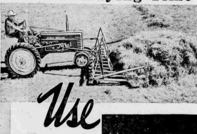
Get your hay up fast and clean with a big-capacity John Deere Tractor Sweep Rake. John Deere Sweeps are ruggedly built yet light in weight. They are easy to attach and detach -your tractor can be made quickly available for other jobs.
