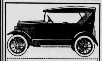
THE body of the NEW OVERLAND Touring Car is made entirely of steel, with baked enamel finish. The hood is higher-body lines are longer-seats are lower and the upholstery removable.
