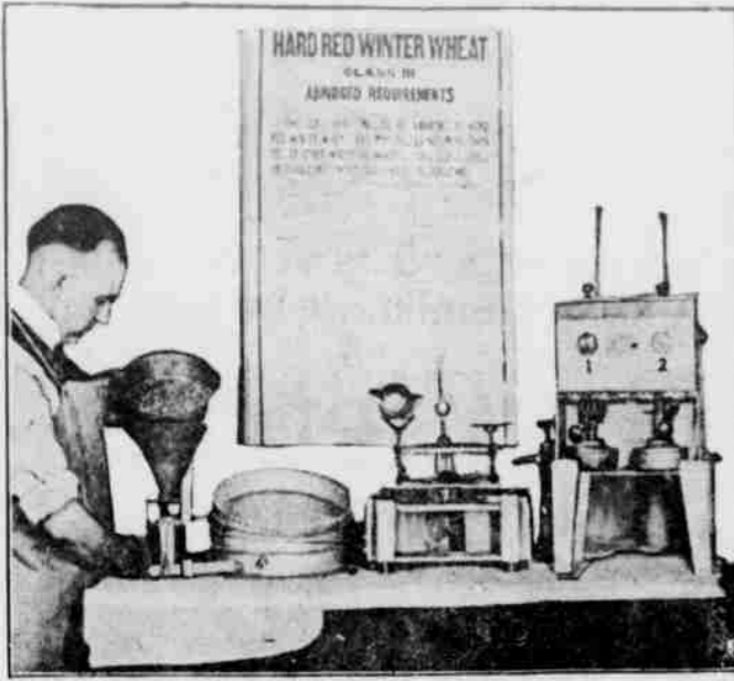
With This Equipment Grain Dealers Can Make All Tests Necessary to Determine the Proper Grade of Grain. From Right to Left Are Moisture Tester, Scales, Sieves, and Weight-Per-Bushel Apparatus.
