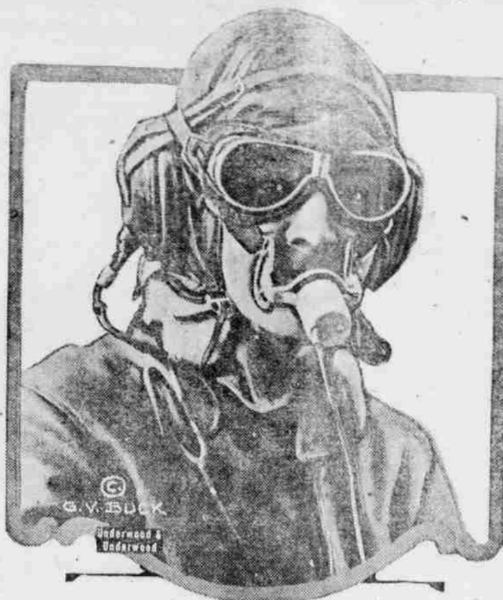
This is the transmitter of the wireless telephone that has been put in successful operation between the land and planes a great distance away. It is worn by the man in the plane.
