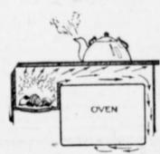
ready for business. The sliding damper regulates the volume of heat going to the ven for fast or slow baking. And the ovens are scientifically constructed to hold an even heat.
