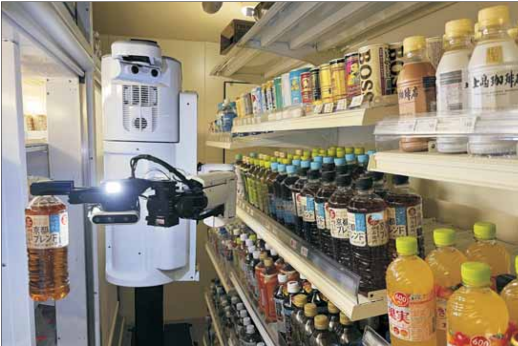
ROBOTIC RESTOCKER. A TX SCARA robot works — stocking drinks in the refrigerated section of a FamilyMart convenience store — in Tokyo. The robot can restock shelves with up to 1,000 bottles and cans per day. (AP Photo/Yuri Kageyama)
