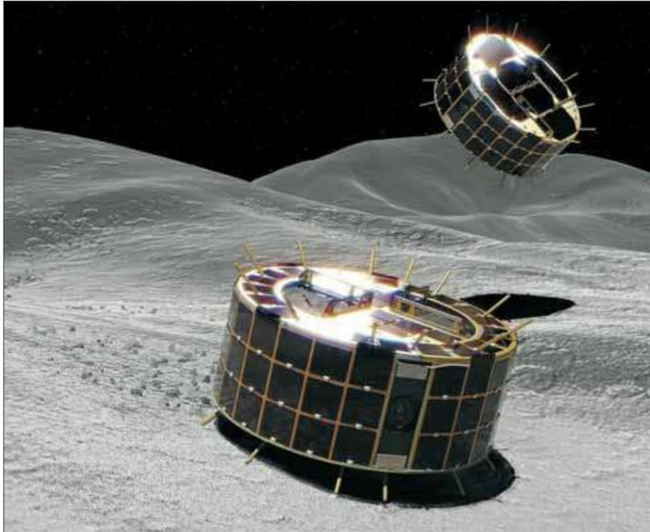
The two rovers, each about the size of a cookie can, are to capture images of the asteroid and measure surface temperatures before a larger rover and a lander are
