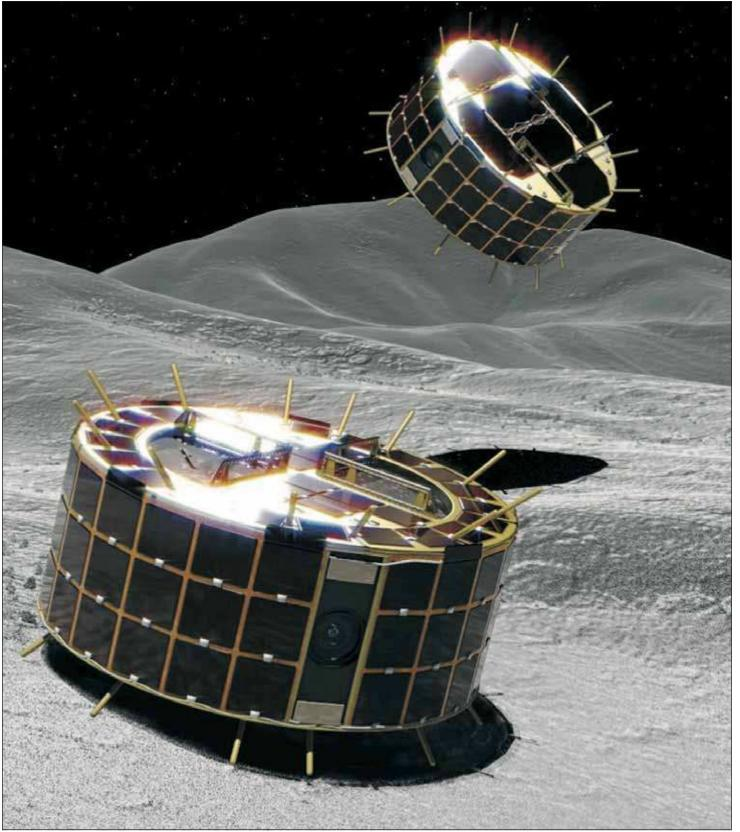
**SCIENTIFIC SPACECRAFT.** This computer graphic image provided by the Japan Space Exploration Agency (JAXA) shows two drum-shaped and solar-powered Minerva-II-1 rovers on an asteroid. Japanese unmanned spacecraft Hayabusa2 approached as close as 180 feet to the asteroid to lower the rovers, waited for a minute, and then rose back to its waiting position about 12 miles above the surface. See story on page 16. (JAXA via AP)
