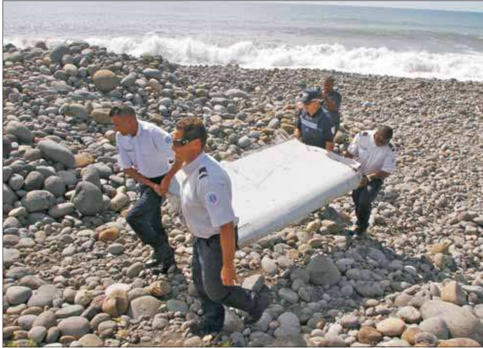
FLAPERON FOUND. French police officers carry a piece of debris from a plane in Saint-Andre, Reunion island. Air-safety investigators, one of them a Boeing investigator, have identified the component as a "flaperon" from the trailing edge of a Boeing 777 wing, according to a U.S. official. Flight 370, which disappeared March 8, 2014 with 239 people on board, is the only 777 known to be missing. (AP Photo/Lucas Marie)
