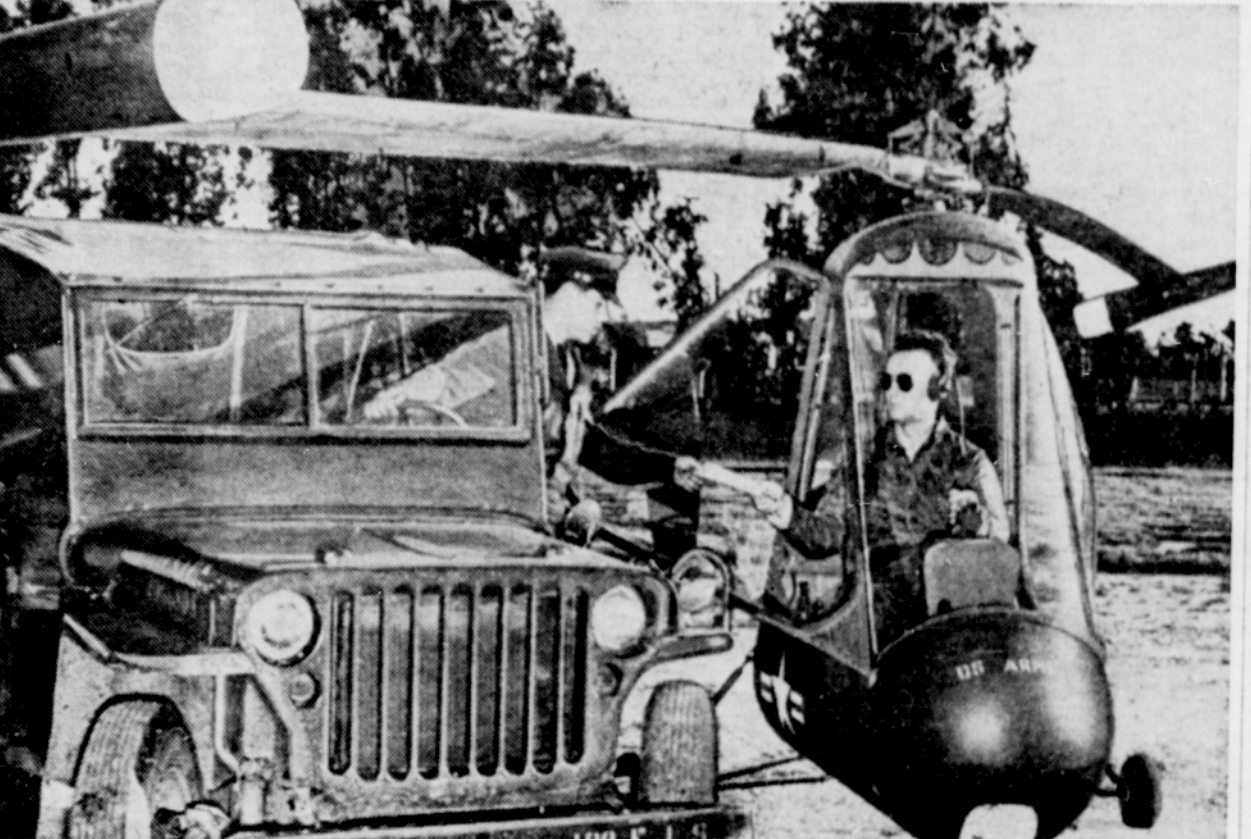
ARMY UNVEILS PINT-SIZE HELICOPTER . . . In Washington, D.C., perched beside a jeep is the XH-26 helicopter announced by the United States army recently. It is designed for air observation as well as evacuation. It can be carried and dropped by a plane by parachute, unpacked and made ready for the air in 20 minutes by two men trained in its operation. It is designed basically as a one-man ship, but can carry two side by side or tandem in twin external litters. The 'copter is powered by two 16-pound pulse jet engines, one on each end of the rotor blades. Top speed is 80 m.p.h., and it can fly for about 90 minutes without refueling, covering a lot of territory.
