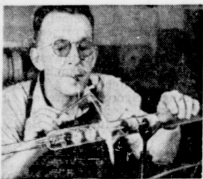
The parts are ready and the column is assembled. Each bubble tray must be spaced and sealed with precision.
