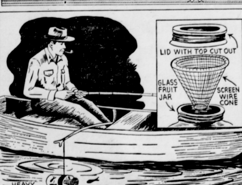
MINNOW TRAP • GLASS FRUIT JAR WITH SCREEN-WIRE CONE FITTED IN MOUTH PROVIDES SUPPLY OF LIVE BAIT. TOP IS CUT FROM LID, LEAVING RIM TO HOLD CONE.
