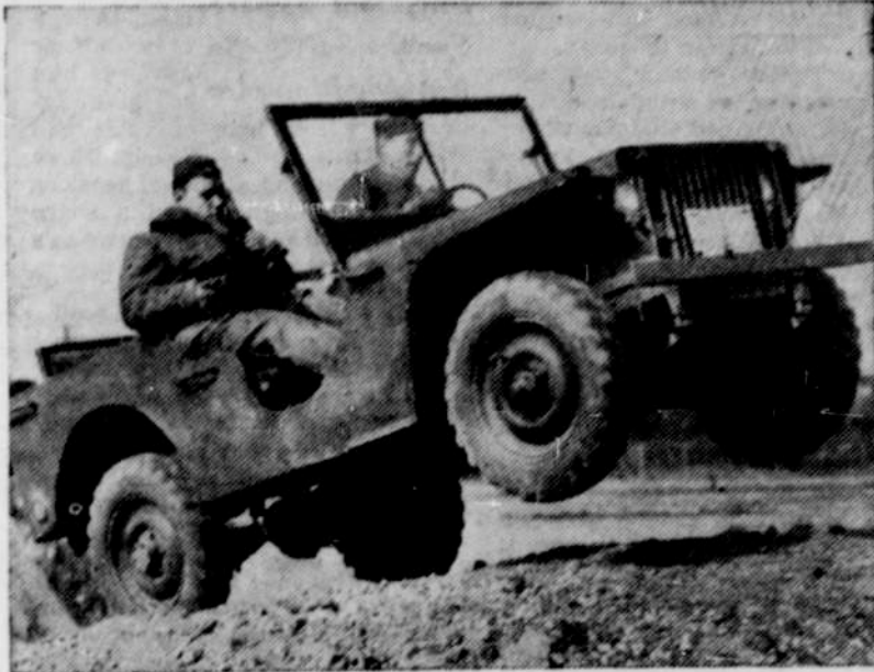
Speed shot at Camp Holabird, Maryland, during tests on new Light Reconnaissance and Command Cars for United States army. They carry machine gun and crew of three men at approximately 60 miles an hour. Can climb steeper hills than tanks.
