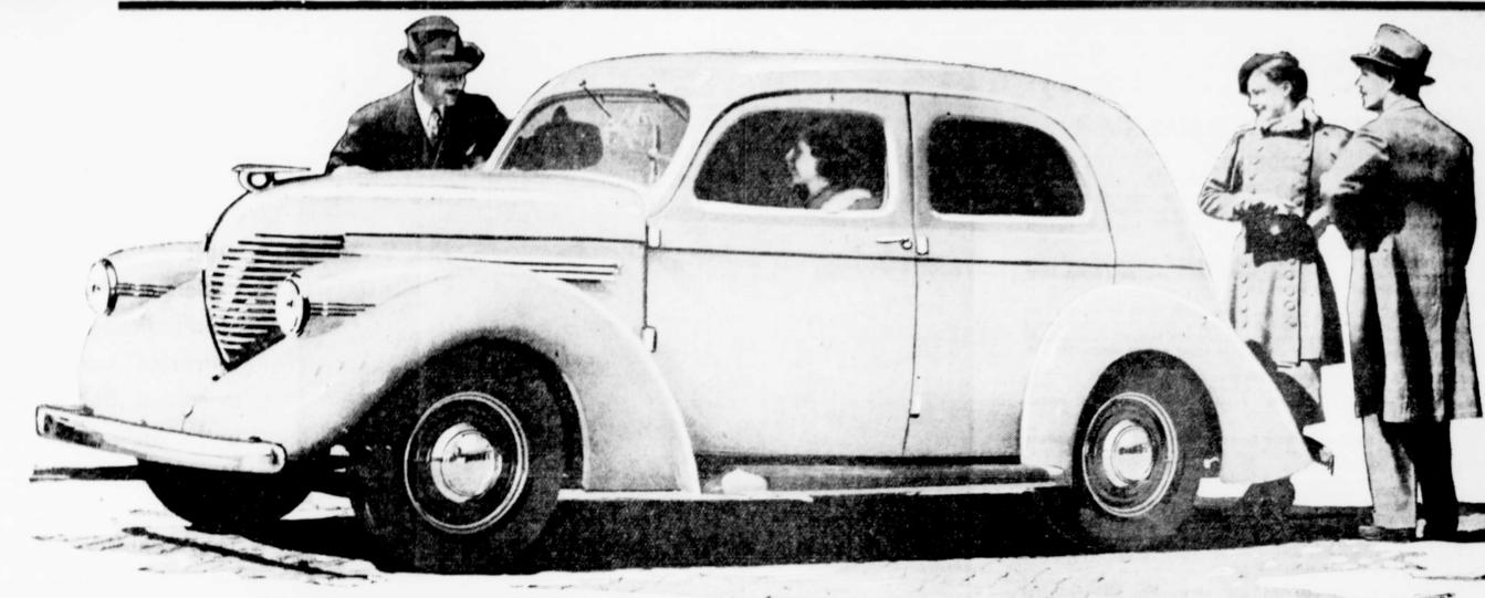
OAD visibility from both front and rear seats, in the sedan models, is as close to 100% as is possible. Glare from approaching headlights, or from following cars in the rear, is reduced to a point where the driver will not be disturbed by reflection in his eyes. This has been accomplished through the pronounced slope of both windshield and rear windows.
