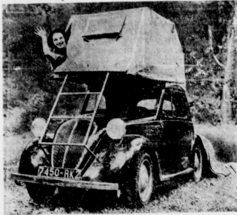
This overnight tent is carried packed up on top of the car and can be unfolded and made ready for a comfortable night in ten minutes. The frame in front supporting the structure serves as a ladder for entering and leaving the tent. The front flap has a zipper at each side.
