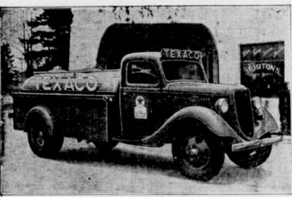
First of the fifteen new tank trucks now under construction at the Beall Pipe and Tank Corporation in Portland for the Texas company. These bodies are being mounted on Ford, Dodge, and International truck chassis and will vary in size from 660 to 1800 gallon capacities.
