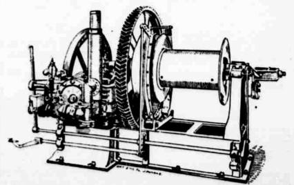
Driving gear, drum shatt, base and all other parts, are extra heavy. Operated by gasoline. By using V tooth gear, extra strength is obtained and noise reduced. Now in Eastern Oregon, near railroad. In good order. Used only few months. No reasonable offer refused. AMERICAN TYPE FOUNDERS CO., Portland, Oregon.
