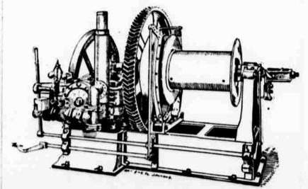
Driving gear, drum shaft, base and all other parts, are extra heavy. Operated by gasoline. By using V tooth gear, extra strength is obtained and noise reduced. Now in Eastern Oregon, near railroad. In good order. Used only few months. No reasonable offer refused. AMERICAN TYPE FOUNDERS CO., Portland, Oregon.
