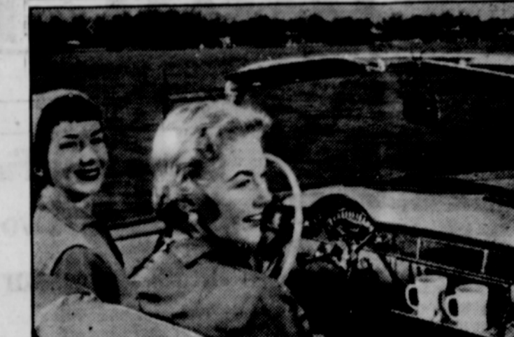
The latest Chevrolets carry an innovation that makes coffee stops more convenient for travelers. The inside of the door to the glove compartment contains two circular wells, forming snug holders for cups. The glove compartment slants downward to prevent spillouts.
