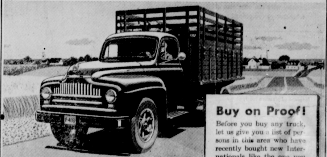
International L-160 series offers GVW ratings from 14,000 to 16,500 lbs., 130 to 172-in. wheelbase.
