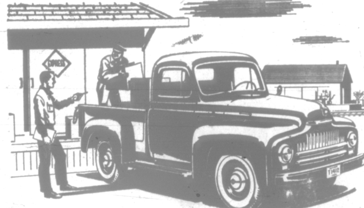
Model L-110, 115-inch wheelbase, 6 1/2-foot pickup body, 4,200 lbs. GVW. Pickups in the L-110, L-120 and L-130 Series include 118, 127 and 134-inch wheelbases, 6 1/2, 8 and 9-ft. bodies, GVW's to 6,600 lbs.
