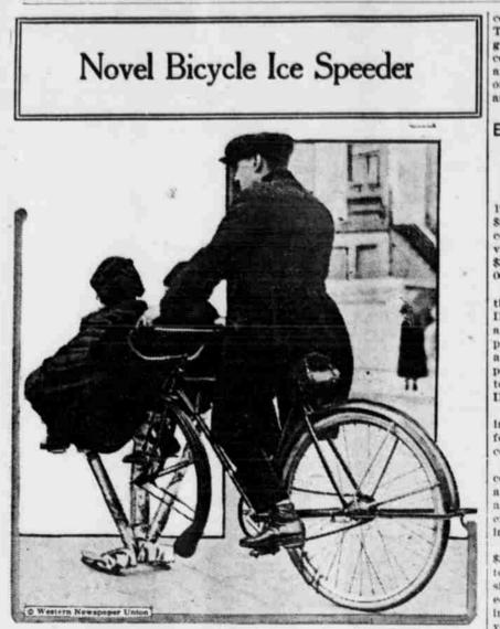
This novel bloycle ice speeder carrying two passengers besides the operator, was made by attaching a fork of wood to the original fork of the bicycle and ice skates fitted on this the same as on the heel of a shoe. The rear tire is non-skid and a piece of chain can be put on just the same as is used on an automobile tire to prevent skidding.
