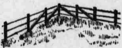
BRACING FOR THE CORNER POST.
