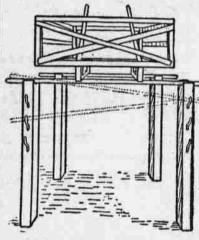
ONE MAN CAN HANDLE BIG BACK. it possible to lift the rack a little at a time by means of the poles, as illustrated by the dotted lines. There is no need of a complicated block and tackle when such a simple device is so effective.-Frank Monroe in Farm and
