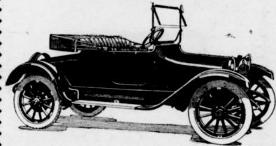
Full floating axle; timken bearings; one man top; electric starter; 35 horse power engine; circulating water pump; real leather up-holstering; electric lights.
