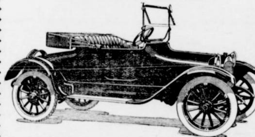
Full floating axle; tim'en bearings; one man top; electric starter; 25 horse power engine; circulating water pump; real leather upholstery; electric lights.
