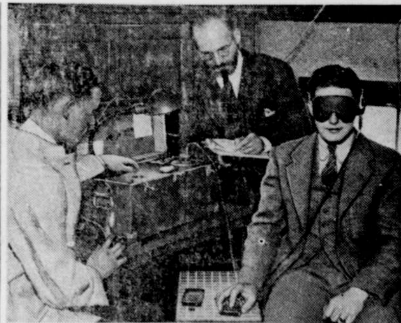
Above: Dr. Laird (center) recording lapses of attention on the part of a blindfolded subject. Dr. Laird's assistant operates the audiometer which generates a tone so faint that the subject can just hear it. The faint tone is constant, but any lapse in attention causes it to become inaudible. Left: In an adjoining room, watching the kymograph as it records lapses of attention. The key from which the subject lifts his forefinger when he ceases to hear the tone, is electrically connected with the kymograph.
