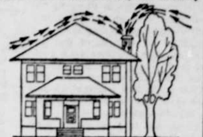
Downdraft—Chimney Too Low. must be both big enough in dimen- sion and tall enough.
