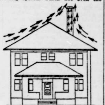
Chimney With Good Draft. most modern vapor-air, warm air cir- culating plant can overcome.
