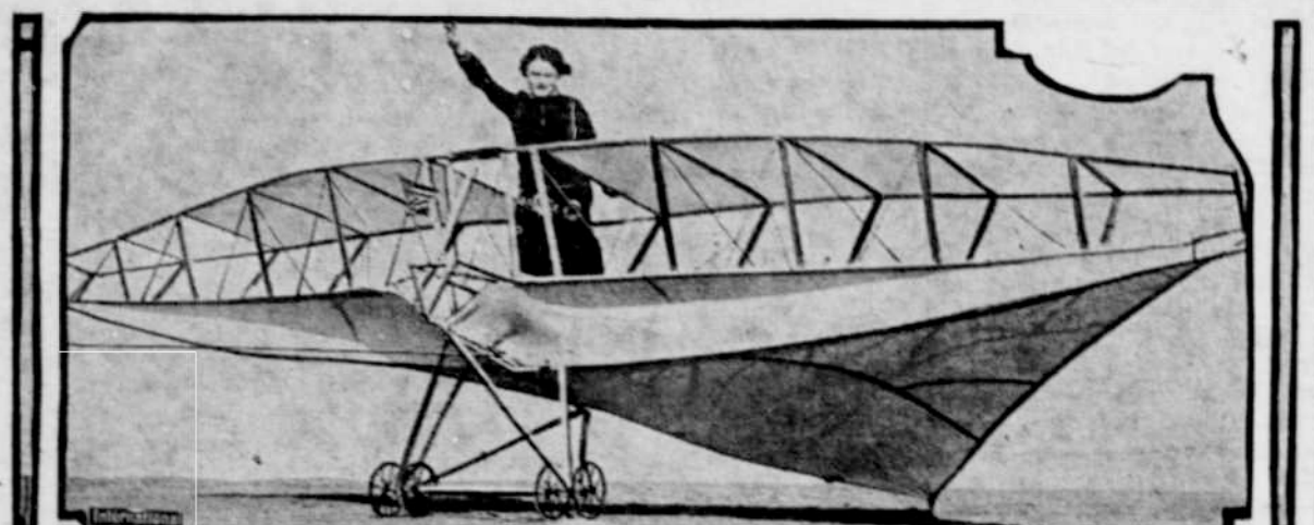
Shown to the public for the first time, after more than 200 trial "flights," this huge passenger-carrying kite is being studied by aero experts at Los Angeles. Invented by George A. Argabrite, who has flown kites since childhood, it has been tested and so far has carried 180 pounds aloft. The photo shows Mrs. Argabrite in the kite.
