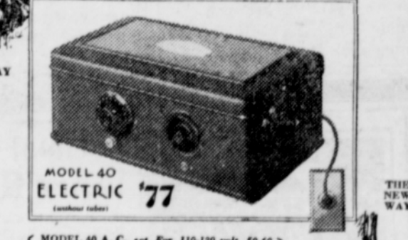
MODEL 40 A. C. set. For 110-120 volt, 50-60 cycle alternating current. Requires six A. C. tubes and one rectifying tube, F77. Also Model 42, with automatic voltage regulator, $86, and Model 44, an extra-powerful "distance" set, $106.
