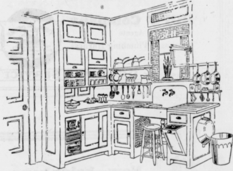
Two-Way or Pass Closet Compactly Arranged With Reference to Dish Washing Closet.
