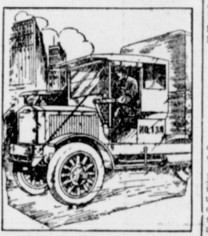
Traffic Signal on a Large Truck is Useful When Making Left Turns.
