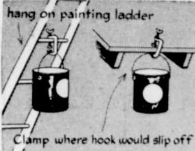
Clamp where hook would slip off
