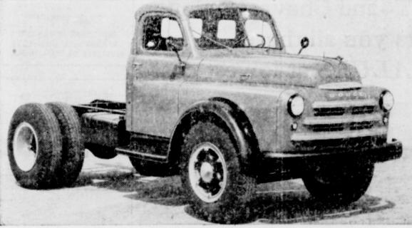
Largest truck offered by Dodge in the new line comprising 356 basic models is this VA-130 model with a rating of 23,000 pounds gross vehicle weight, and 40,000 pounds gross combination weight. This model is offered in five wheelbases. It has a 331cubic-inch engine, sodium-cooled exhaust valves,
