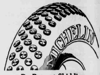
Do Prevent Skidding Rubber Traction Surface Protected and Reinforced by Tough, Flexible, Non-puncturing Leather Tread, An Integral Part of the Tire and Not An Attachment. Firmly Imbedded Hardened Steel Studs Do Prevent Skidding.
