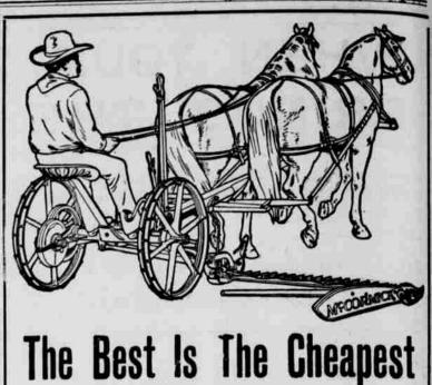
In the McCormick mowers, you get the lightest running and most durable machine made. All of the principal bearings in the McCormick are equipped with rollers which reduce the friction to a minimum. There is no side draft to the McCormick mower, and you do not have to back your machine to start it in heavy grass. The McCormick costs no more than other sta-dard machines, and is sold on easy terms. Call and let us show them to you.
