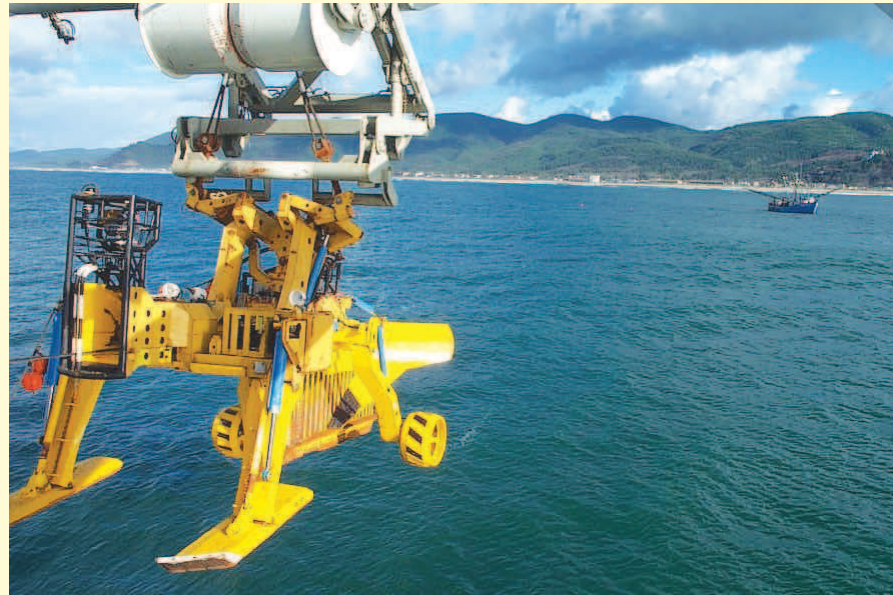
Above: Fishing Vessel Ken & Al, based in Warrenton, serves as patrol off Rockaway Beach while operators prepare to lower a seaplow that will dig a trench for a new cable.
