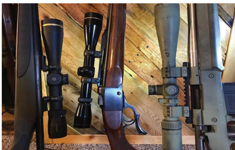
Scopes with adjustable turrets may be big and bulky but can help with long-range accuracy.
