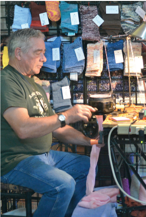
Eagle file photo Gary White of Socks of Fun in Oregon City owns an antique sock machine. The machine, made in Pennsylvania about 100 years ago, was used to make socks for soldiers during World War I and World War II.
