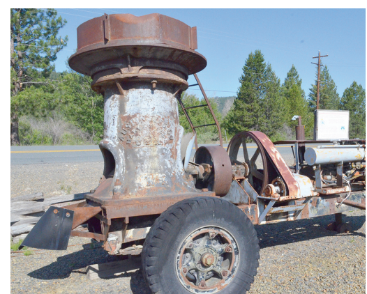
This machine on display at the Cracker Creek Museum of Mining in Sumpter combined a 1900-era cone crusher with a 1950s-era gasoline engine.
