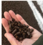
Torrefied Wood Pellets
