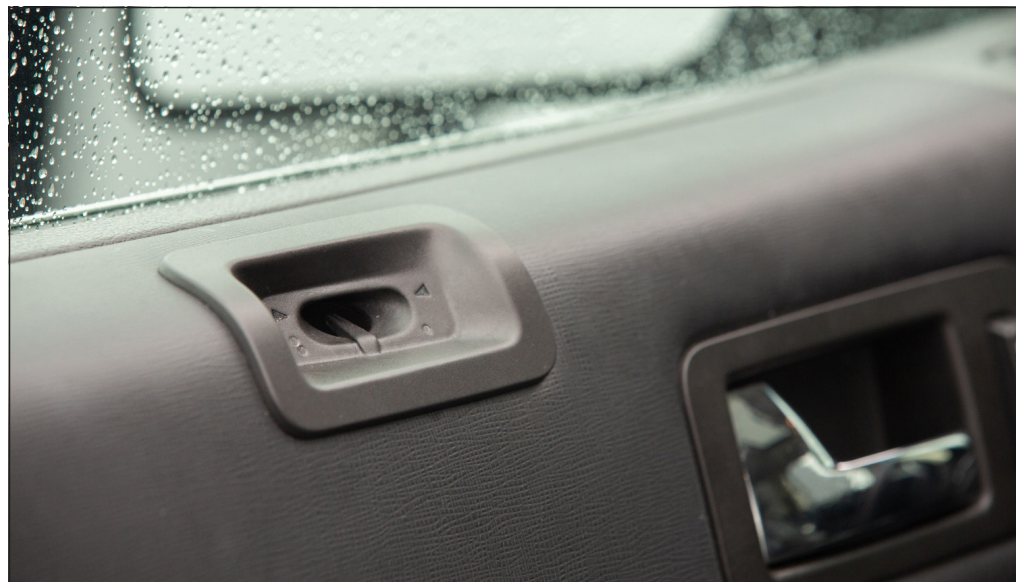
A universal ignition interlock used to combat drunken driving. Unlike ignition interlocks in use today, mostly for people charged or convicted of drunken driving, the new technology would be built into the vehicle.
